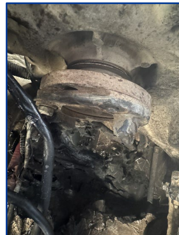
Transfer case where the front drive shaft broke off.
